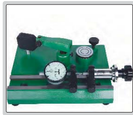
inspect accuracy of dial indicators (range 0-25mm)
