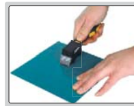
step 1: make grid cutting on surface
